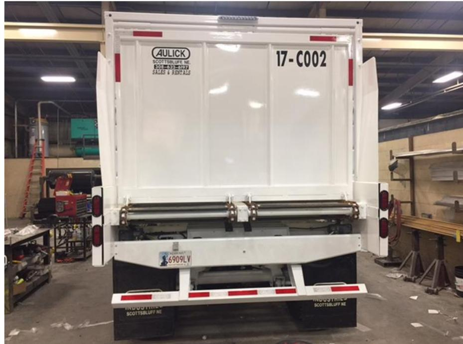
**THE REAR SHAFT IS HELD IN PLACE BY UHMW BLOCKS. EACH BLOCK HAS A GREASE ZERK ON IT THAT SHOULD BE GREASED DAILY.**
