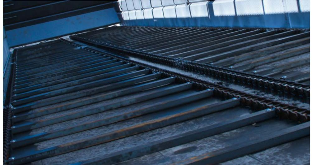
**THE FLOOR CHAIN IS D88C CHAIN WITH STEEL CROSSBARS HUCKED, NOT WELDED, FOR EASY REPLACEMENT WHEN NECESSARY.**
