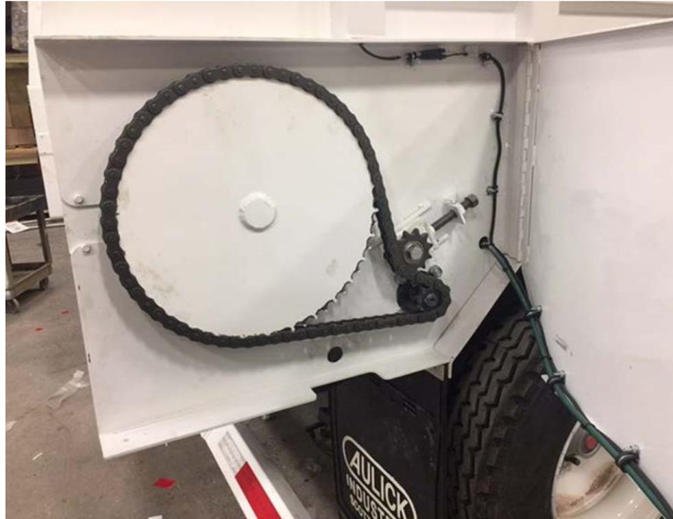
THE DRIVE CHAIN TENSION SHOULD BE CHECKED DAILY. THERE IS ONE ON EACH SIDE OF THE TRAILER. TO TIGHTEN THE TENSION, LOOSEN THE IDLER SPROCKET BOLT AND JAM NUT ON THE TENSION BOLT.
